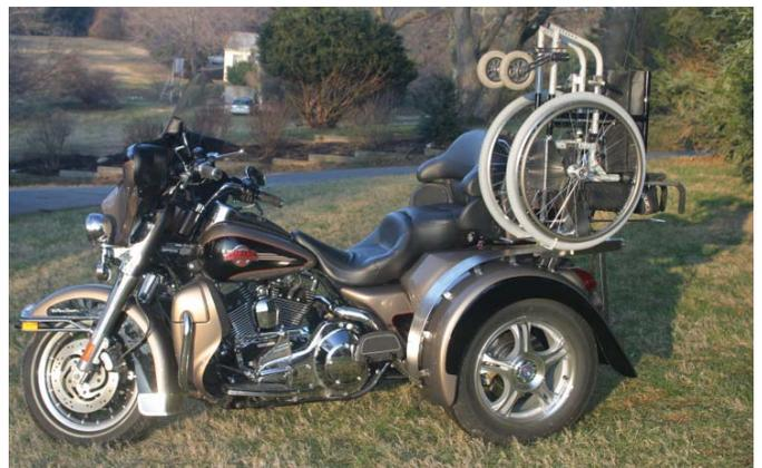
*Here is a wheelchair lift on a custom trike. The wheelchair is attached to an arm on a track that lifts it onto the fender. The lift gives riders wheels on their bike or in their chair and is the product of The Freedom Track, [www.freedom-track.com](http://www.freedom-track.com).*
