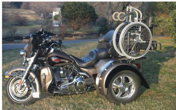
*Here is a wheelchair lift on a custom trike. The wheelchair is attached to an arm on a track that lifts it onto the fender. The lift gives riders wheels on their bike or in their chair and is the product of The Freedom Track, [www.freedom-track.com](http://www.freedom-track.com).*
